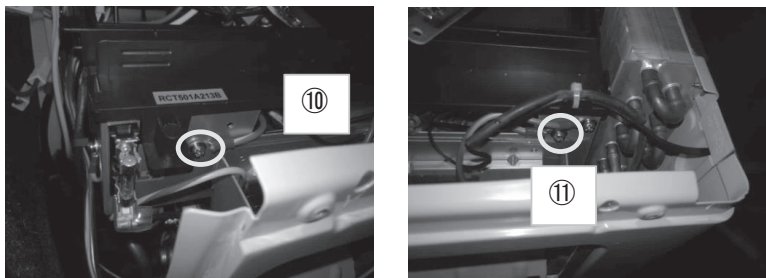
Fig.5 Earth cable of control box
