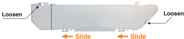
No need to remove screws
